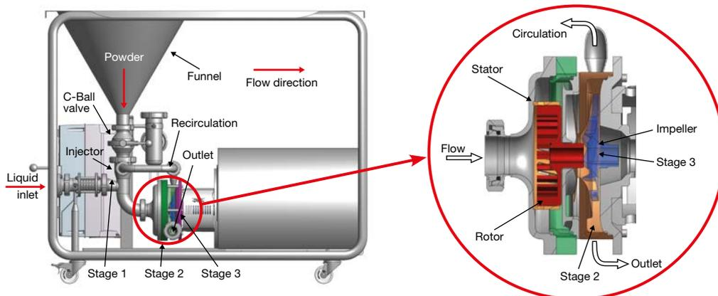
**Highly efficient preparation of concentrated pectin solution**
