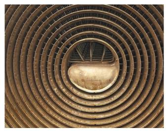
Detail of a spiral heat exchanger before Alfa Laval reconditioning.
