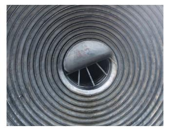
The same Alfa Laval spiral heat exchanger after reconditioning.
