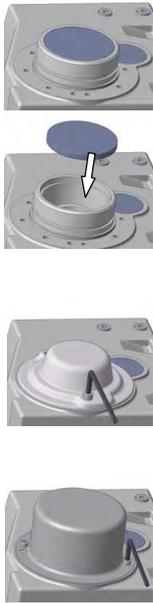
Figure 3-12: Fitting the covers, Option SH, Option H, and Option H66
