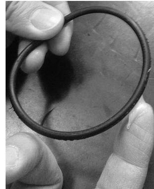
Figure 6, Greasing O-ring
