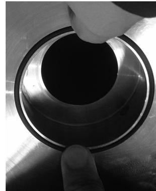
Figure 7, Inserting O-ring
