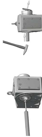
Figure 3-5: Removing the factory-fitted closing cap
