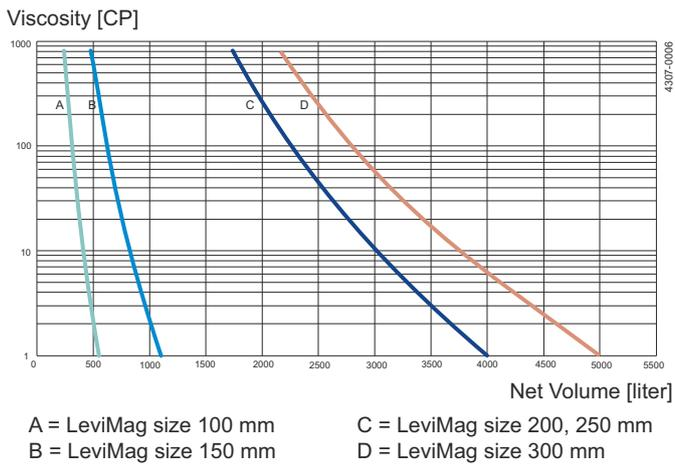
Figure 5. Duty Level 3: Mixing Volume vs. Viscosity
