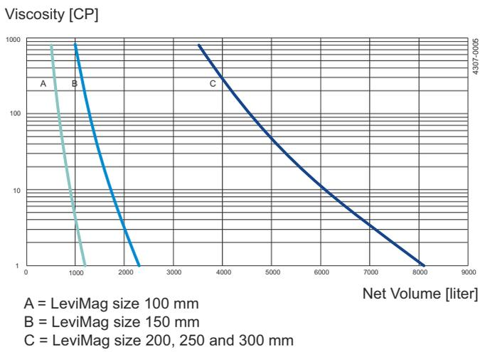
Figure 4. Duty Level 2: Mild blending Volume vs. Viscosity
