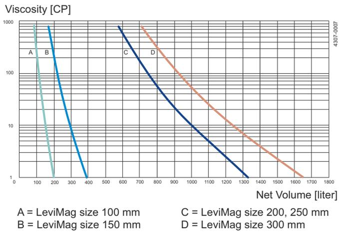
**Figure 6. Duty Level 4: Powerfull mixing Volume vs. Viscosity**
