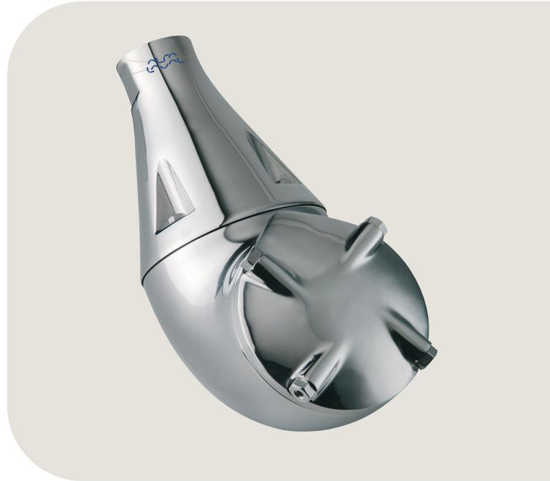
the tank. The nozzles rotate around both the horizontal and vertical axes in a 360° movement. This three-dimensional jet rotation enables the jets to reach the entire tank volume, providing fast, efficient mixing of the injected liquid, gas or powder without requiring batch rotation.
