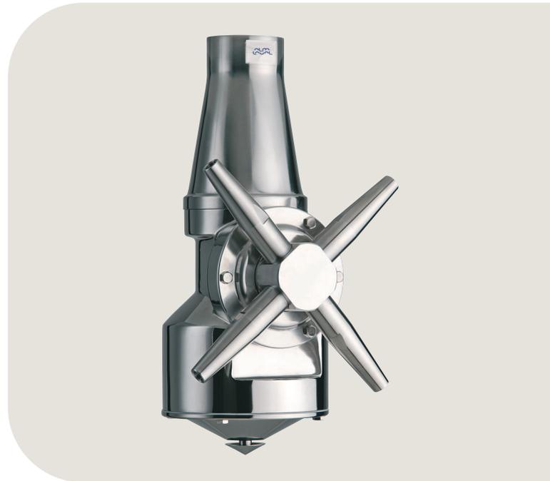
liquid in the tank. The nozzles rotate around both the horizontal and vertical axes in a 360° movement. This three-dimensional jet rotation enables the jets to reach the entire tank volume, providing fast, efficient mixing of the injected liquid, gas or powder without requiring batch rotation.
