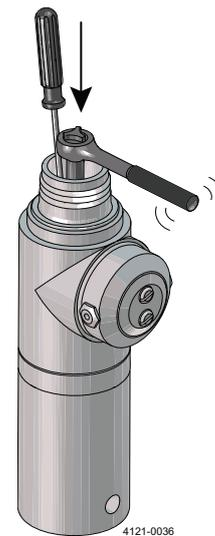
7. Test for proper assembly by turning the impeller with a pencil or screwdriver. The input shaft should turn very easily and the impeller vanes must not strike the stem wall.
