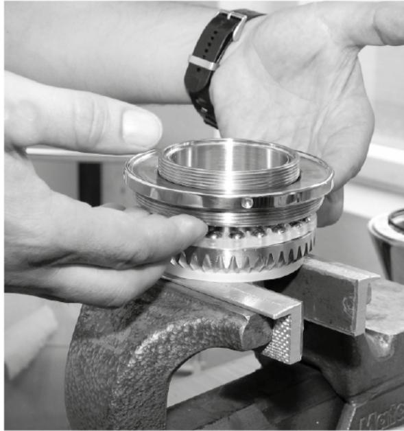
5. Preparation of O-rings (6 and 7) before mounting: Dip the O-rings in water. If water is not used then be very careful about how the O-rings behave when screwing the cone (1.1.) onto the stem.
