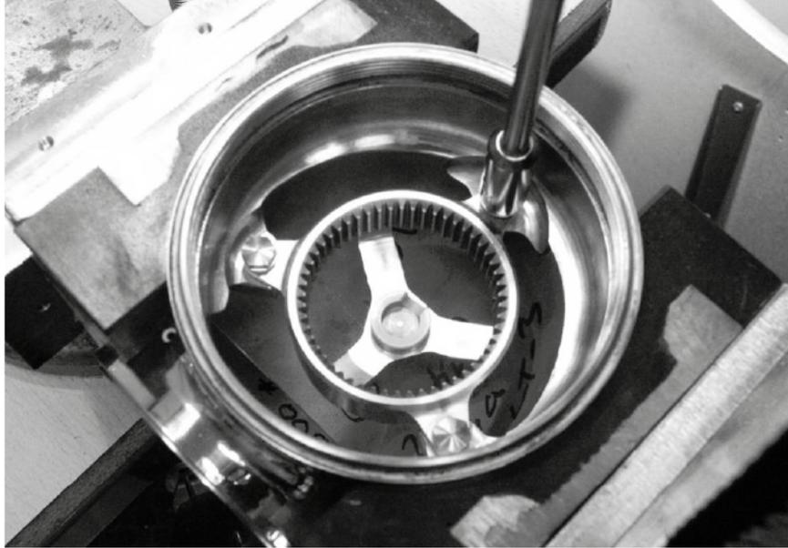
9. Remove the assembled gear ring (13.2) from the body and remove the 6 seal rings (13.4)
