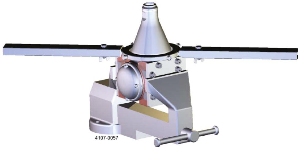
3. Tighten the 4 screws (by hand only) symmetrically into the 4 hygienic recesses in the stem nut (4).
