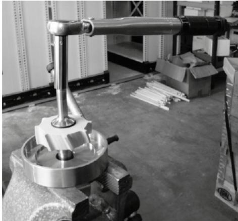
5. Screw the shaft end (Pos. 3.4) into the turbine shaft (Pos. 3.1) using the torque wrench (TE81B156) and NV9 spanner socket (TE81B158). Tighten with torque of 10-12 Nm.
