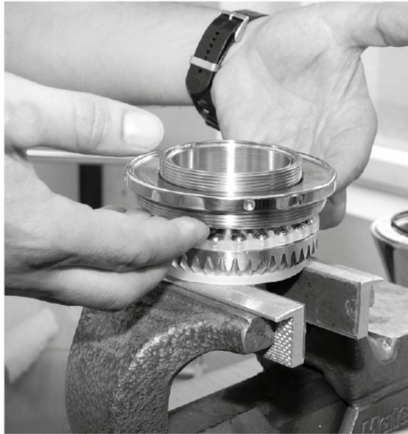
5. Preparation of O-rings (Pos. 6 and 7) before mounting: Dip the O-rings in water. If water is not used then be very careful about how the O-rings behave when screwing the cone (Pos. 1.1.) onto the stem.
