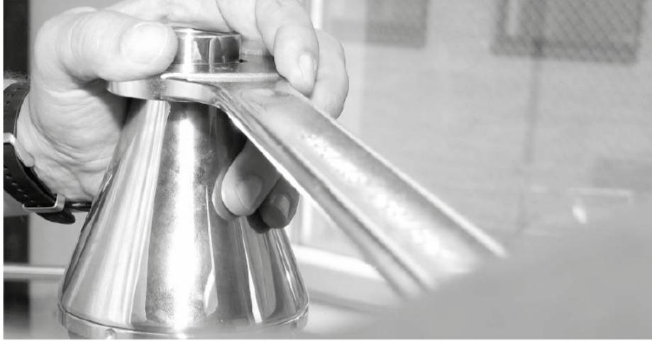
4. Loosen the cone (Pos. 1.1) by hand while lifting the cone vertically and finally remove the cone (Pos. 1.1)
