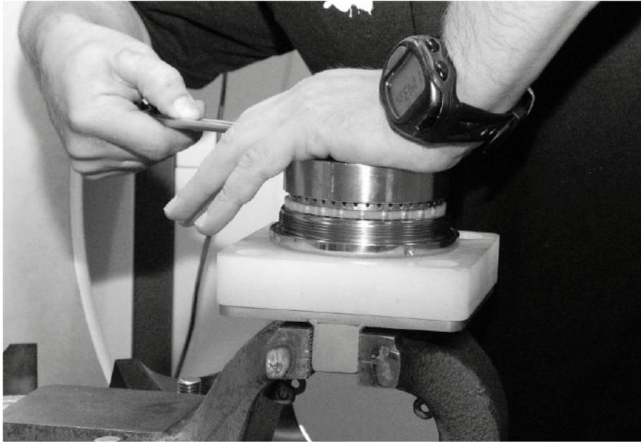
12. Check that the hub nut (Pos. 15) can rotate freely and that O-rings inside are mounted correctly (Pos. 16 and 17).
