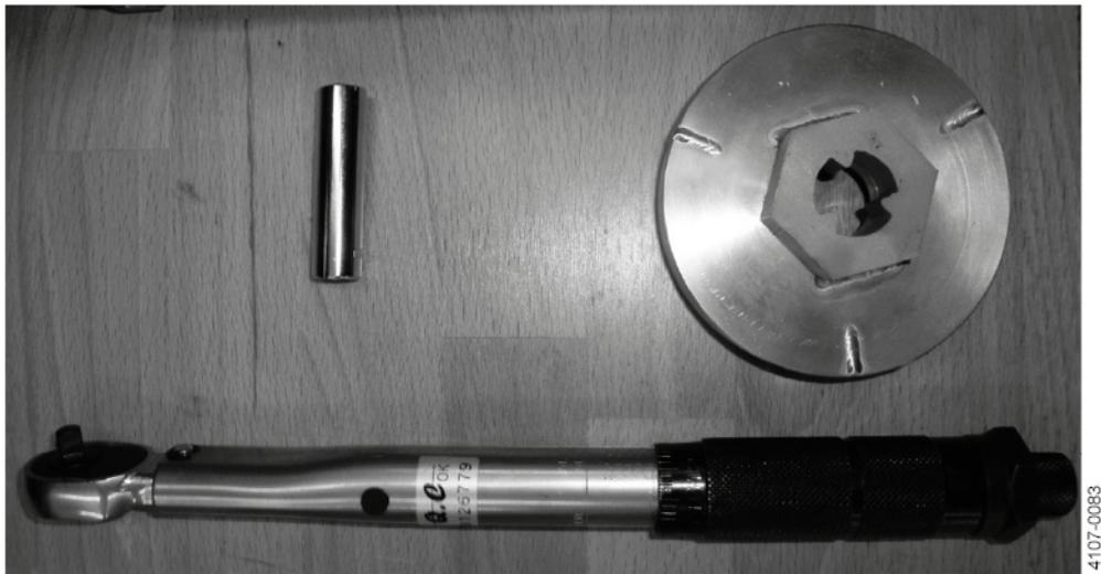
1. Mount the impeller turbine fixture (TE20J392) in bench vise. Loosen the shaft end (Pos. 3.4) using the torque wrench and NV9 socket long (TE81B156 + TE81B158) and unscrew with hand.
