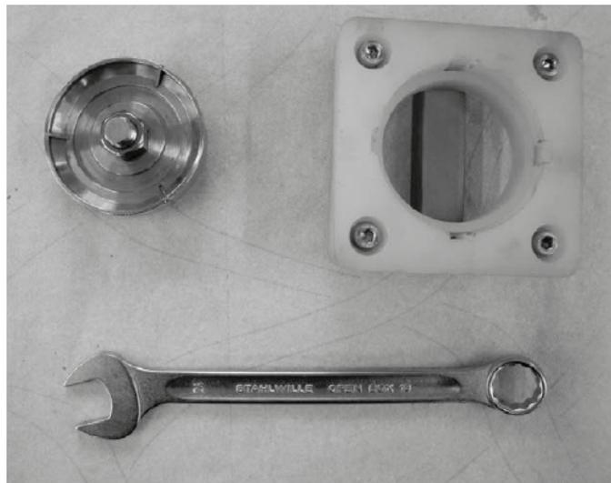
1. Place the fixture for nozzle (TE20J366) into the bench vise and secure it
