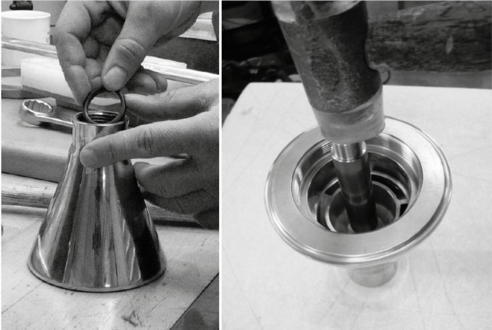
10. Push out bushing (Pos. 1.2) from the top of the cone using the drift (TE81B139)
