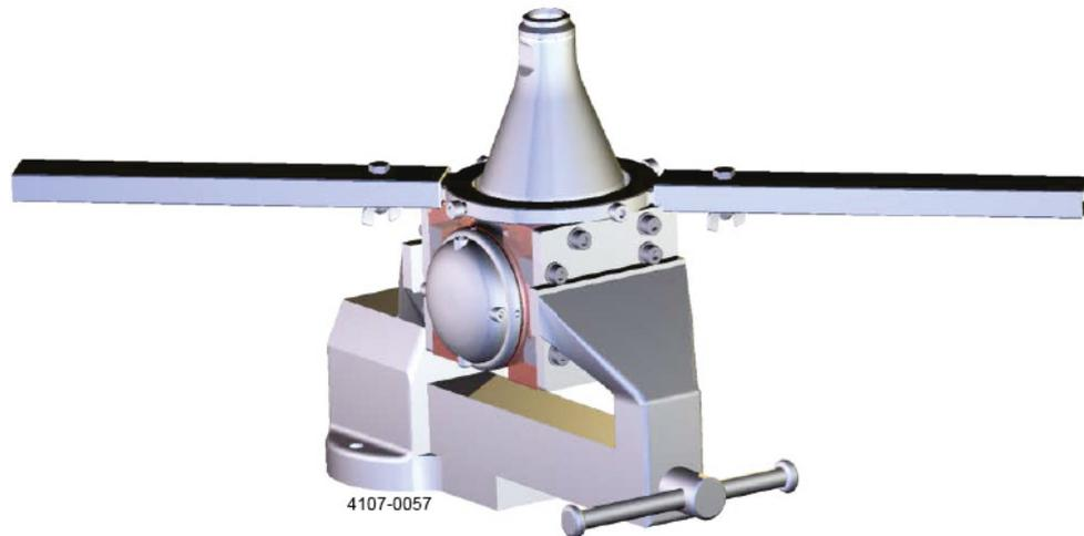
3. Tighten the 4 screws (by hand only) symmetrically into the 4 hygienic recesses in the stem nut (Pos. 4).
