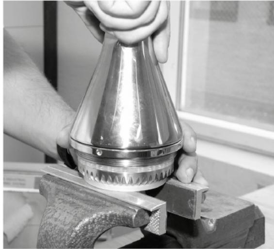
10. Tighten the cone (Pos. 1.1) using the ring key spanner (TE81B141 or TE81B159) until you feel a stop and then tighten it a bit more. The stop you feel is two surfaces connecting.
