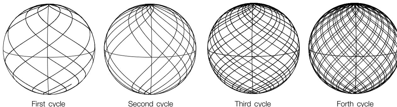
The number of cycles needed to perform a proper cleaning depends on type of soilage, position of the tank cleaning machine, cleaning procedure, cleaning temperature and cleaning agent.
