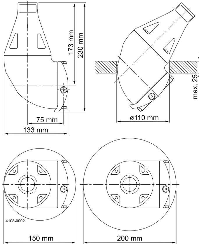
Minimum required passage:  $\varnothing 110$  mm (4.33 inch) at flange thickness 25 mm (0.98 inch). Otherwise  $\varnothing 150$  mm (5.90 inch).
