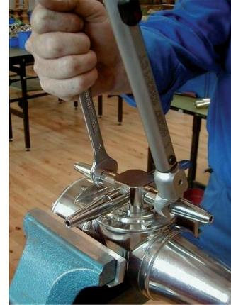
3. Check that the machine is in operating condition by inserting 3/16" hex Screwdriver (tool No. TE134A) in screw in top of Turbine shaft and easily turn Turbine shaft clockwise. If any resistance is recognised, the machine should be disassembled to localise the cause.
