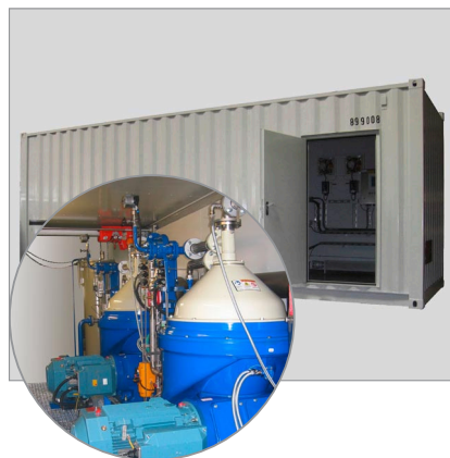
Fig. 10 and Fig. 11. FALCON 25-200 module containerized for arctic conditions.
