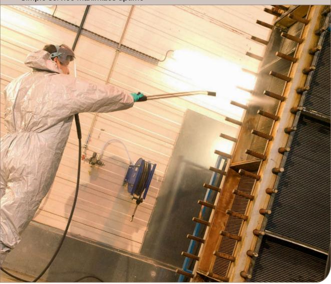
Compabloc is a breakthrough plate heat exchanger design that combines several major process advantages in one compact unit. The all-welded plate pack eliminates gaskets between plates, which makes it possible to operate with a wide range of aggressive media, high temperatures and high pressures. The corrugated plate patterns minimize fouling and make
